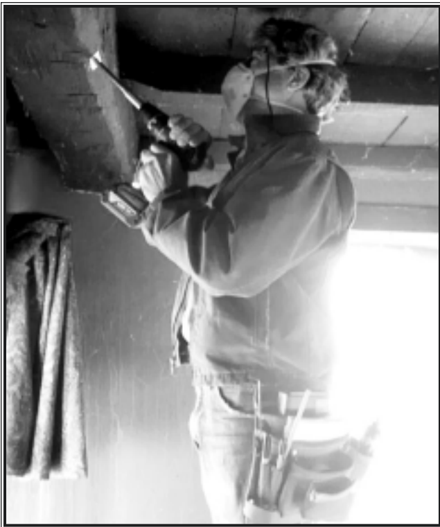
Core samples were taken earlier in the year to determine the age of a home at 24 Griffin Road that was slated to be demolished. Photo courtesy of Ann Chiampa.
